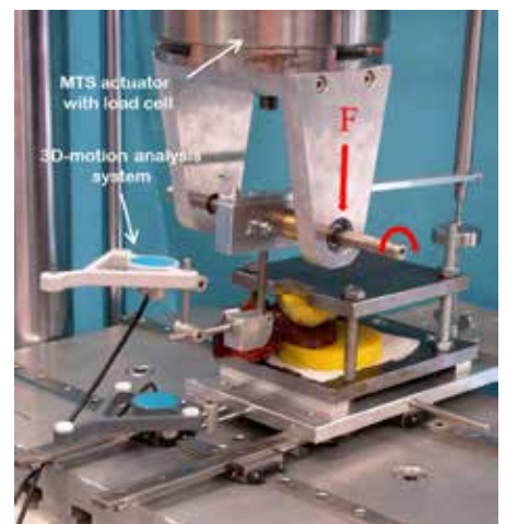
Fig.2: In vitro test set-up used to apply physiological loading to pedicle screws and provoke screw loosening. Red arrows show the load application and the pivot axis to allow a tilting motion of the screw in the vertebral body.
