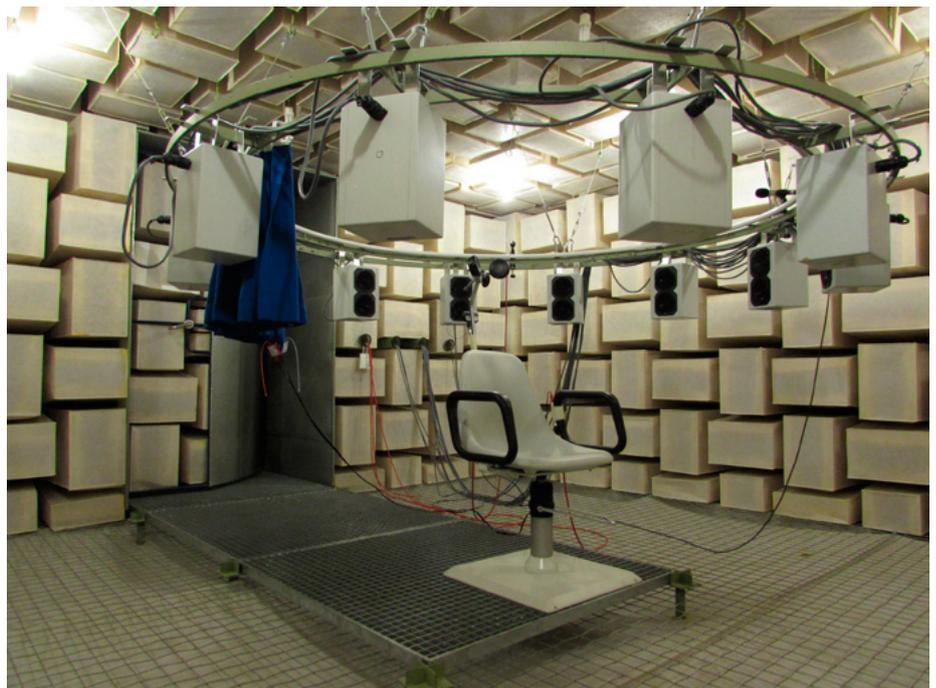
*Fig. 1: The anechoic chamber is a special room for high-precision psycho-acoustic measurements. The background noise level in the chamber is less than -10 dB Hearing Level at all frequencies between 16 and 20,000 Hz. Loudspeaker boxes are mounted in a horizontal plane for testing a person’s sound source localization skills.*
