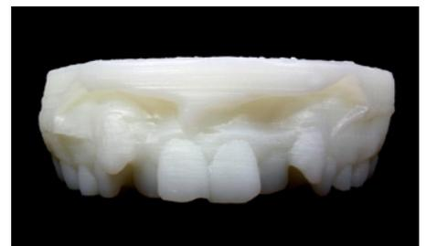
Fig. 2: Model printed by Formlabs Form 1
